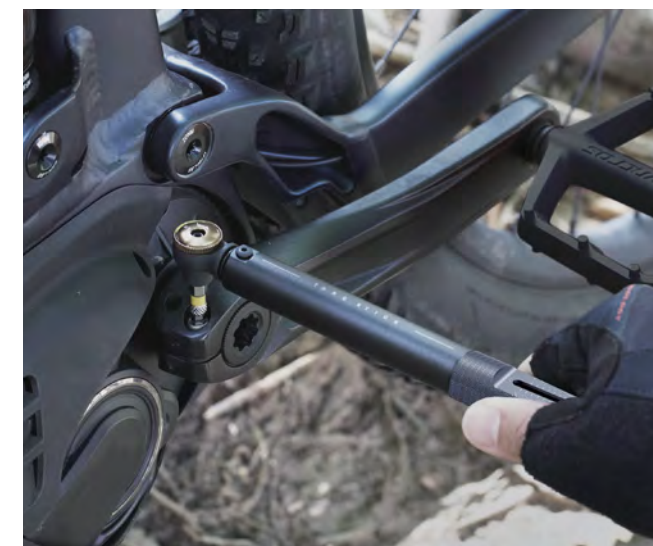
Torque wrench with adjustable preset range of 4 - 20Nm
