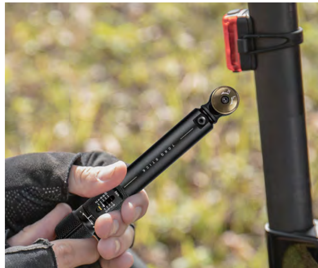
Torque wrench with adjustable preset range of 2 - 10Nm
