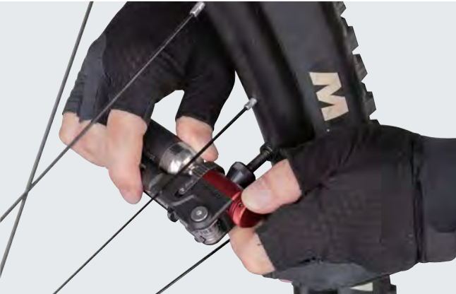
4. Release Flow Control Knob to control inflation speed
