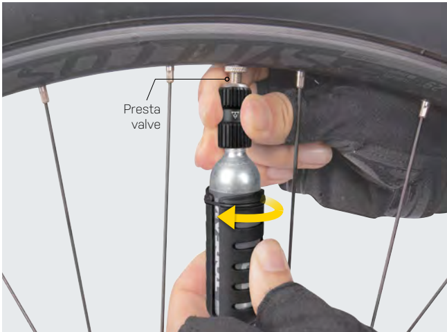
2. Hold Nano AirBooster and unthread CO 2 Cartridge 1/2 turn to inflate tire
