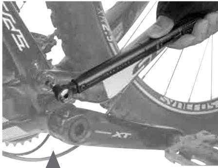
When the preset torque value is reached, an audible "CLICK" sound will be heard. Stop applying torque to the fastener.
