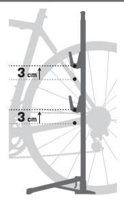
Lift bike onto Folding Hooks then fine tune height adjustment as necessary.
