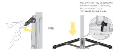
2 Close hook and slide to adjust to proper height. Open hook to lock in position.
