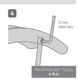
Tighten all bolts after installation is complete.
