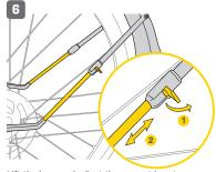
Lift the lever and adjust the support legs to proper length on both sides.
