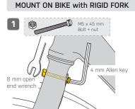
Hold the bolt nut and tighten the bolt at the same time.
