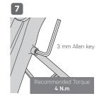
Tighten all bolts after installation is complete.
