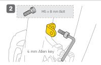
Install the L shape Fork Adapter as shown.
