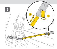
Lift the lever and adjust the support legs to proper length on both sides
